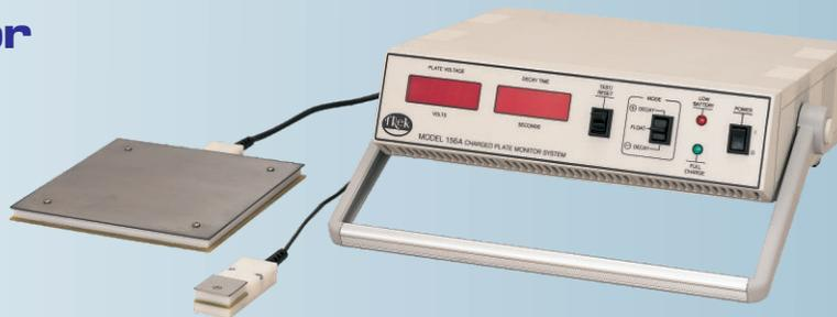
The Model 156A tests the efficiency of an ionizer's ion production by timing how long it takes air ions produced to discharge a floating plate that has been pre-charged to either a positive or negative value. The Model 156A also tests the balance between positive and negative air ions by measuring the offset voltage generated on a floating plate due to an imbalance of positive and negative air ions impinging on the plate from the ionizer.
