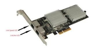
There are two LEDs next to either side of the Ethernet port on the network card.
