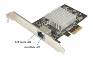
There are two LEDs at the two top corners of the Ethernet port on the network card.
